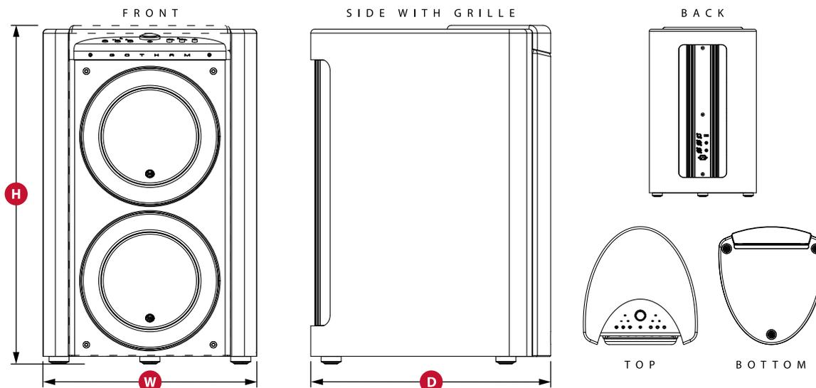
\* All height dimensions include feet, depth dimensions include grilles.
