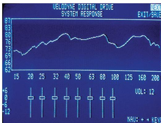
**Fig.4** Quad ESL-989 output with two JL Audio Fathom f113s after running ARO, in-room response (25dB vertical range).
