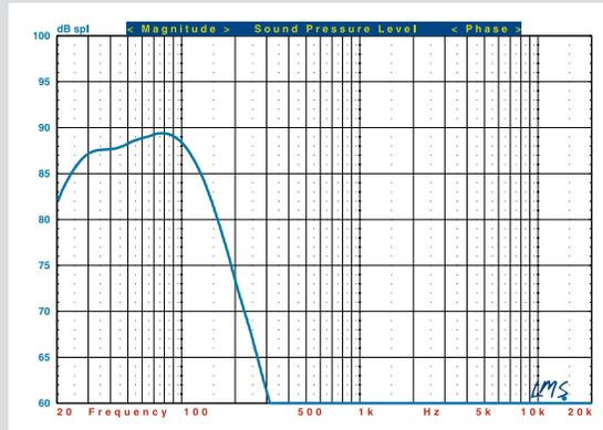
**e110 (blue)** Close-miked response, normalized to the level at 80 Hz: lower -3 dB @ 26 Hz, -6 dB @ 21 Hz, upper -3 dB @ 119 Hz with Crossover switch set to Off.—MJP
