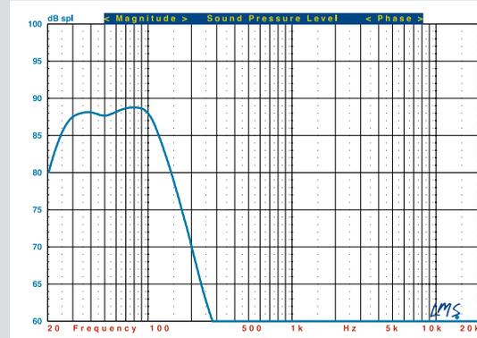
**DOMINION D110 (blue)** Close-miked response, normalized to level @ 80 Hz: lower -3 dB @ 25 Hz, -6 dB @ 22 Hz, upper -3 dB @ 115 Hz with LP Filter switch set to Off.—MJP
