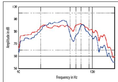
**Fig.1** (top) JL Audio E-Sub e110, in-room response of individual subwoofers (left channel, blue, right, red) and summed response (green) (5dB/vertical div.). **Fig.2** (bottom) JL Audio E-Sub e110, in-room summed response before (blue) and after (red) calibration by Audyssey (5dB/vertical div.).
