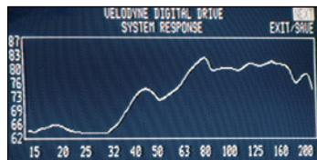
Fig.1 Quad ESL-989s, no subwoofer, in-room response, 20Hz–200kHz (25dB vertical range).
