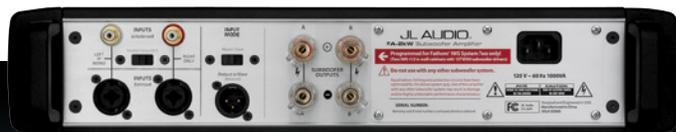
● The amp features balanced or unbalanced inputs.
