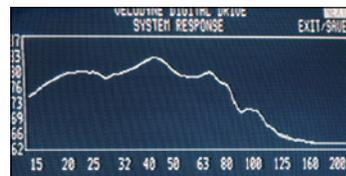
Fig.2 JL Audio Fathom f212s, uncorrected in-room response (25dB vertical range). Notice 50Hz peak.
