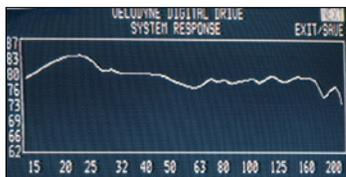
Fig.3 Quad ESL-989 in-room response with two JL Audio Fathom f212s after running ARO, and setting low-pass filter of left Fathom f212 to 40Hz (25dB vertical range).
