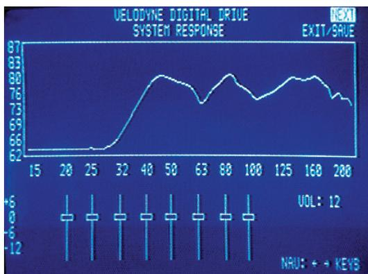
**Fig.1** Quad ESL-989 frequency output, 20–200Hz, no subwoofer, in-room response (25dB vertical range).
